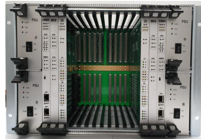
Figure 4: IP control unit for Light Signal
