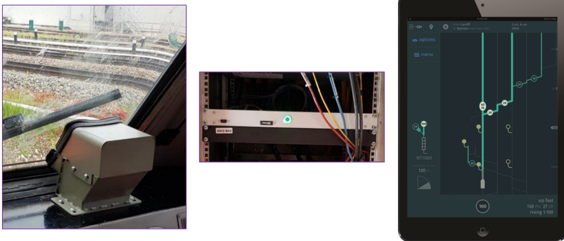
Figure 8: VTPS camera installation (left), VTPS 1U rack processing unit (centre), Driver Support System tablet application (right)
