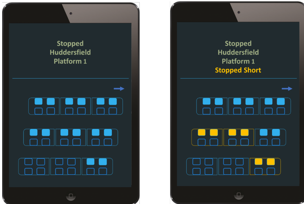
Figure 10: Driver display for Automatic Selective Door Opening using virtual balises
